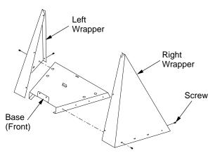
Figure 2 - Attaching Left and Right Wrappers to Base
